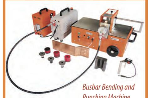
Busbar Bending and Punching Machine
